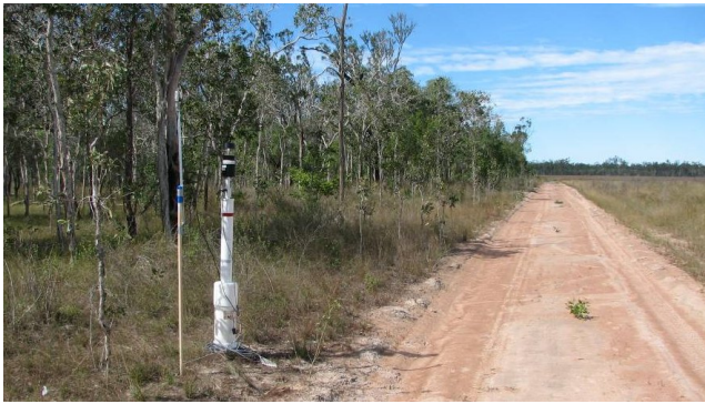
Figure 4: TACMET-Augmented Sensor Agent at the Talisman-Saber Drop Zone (Note the “high-tech” broom-handle antenna mast to the left of the sensor.)
